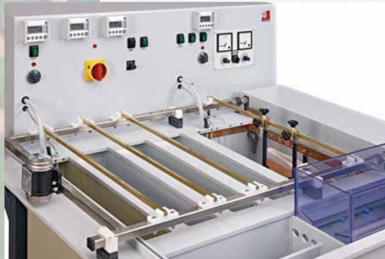
The modular design of the systems provides the ability to integrate additional processes into the system concept: desmearing, blackening, tin stripping, resist stripping, immersion tin and organic protective coating (OSP), immersion nickel / gold, immersion silver, electroplated nickel / gold. The treatment and rinsing tanks are optimally fitted with high-quality facilities and system components which guarantee an optimal result for printed circuit board.
